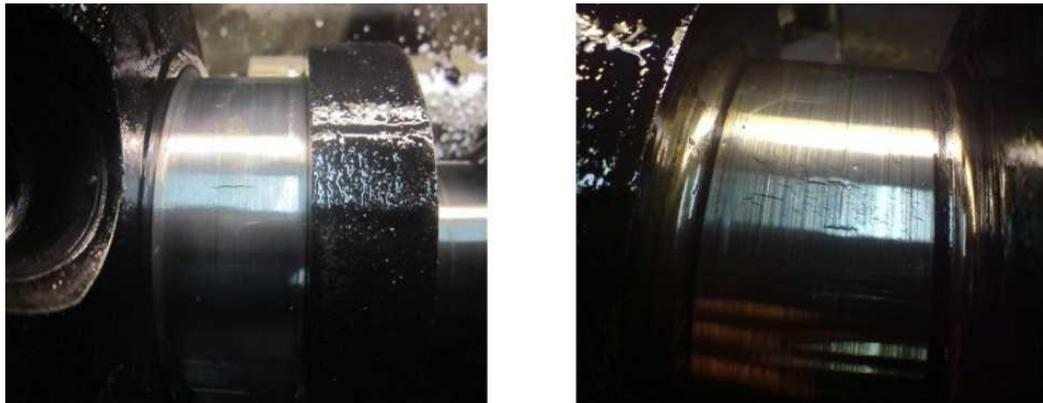
*Fig. 3. Fatigue cracks on the shaft neck*
