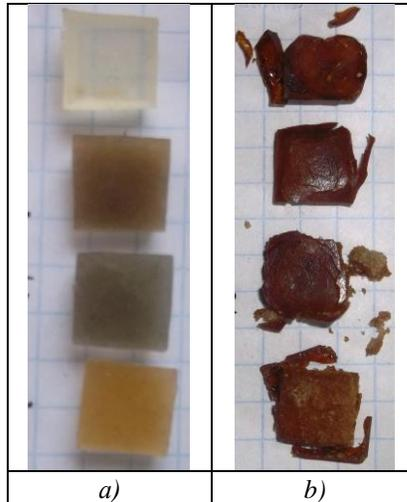
Fig. 2. Type of composites with 50 wt% of sand taken for experiments:
